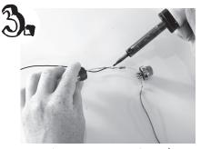
Solder the resistor to one of the black wires. Solder the other end of the resistor to the uppermost leg on the right side. Solder a new black wire to the middle leg on the right side.
