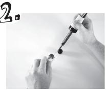
Place the MQ4 sensor down with the feet up and the sticker on the top. Solder the red wire from the battery holder to all the left feet.
