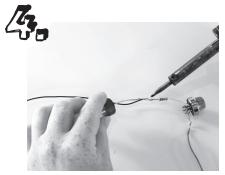
Solder the blue wire to the bottom leg on the right side. Solder the other end of the blue wire to the 2K ohm resistor and then to the "+" side of the VU meter.
